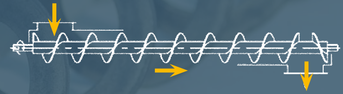
3 Left-hand ribbon flight, electric motor clockwise rotation, for material flow direction, please see the diagram
