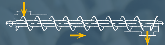
2 Right-hand ribbon flight, electric motor counterclockwise rotation, for material flow direction, please see the diagram
